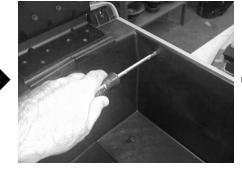
**STEP 4:** With a screwdriver remove the four screws that are found around the top edge of the storage bucket.
